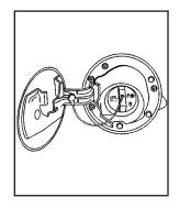
The tethered fuel cap is located behind a hinged fuel door on the driver's side of the vehicle.
